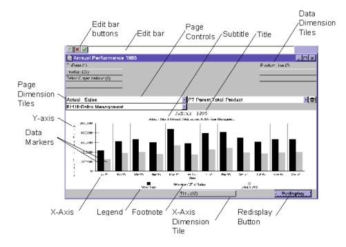
The following illustration shows a vertical bar graph with elements of the graph window labeled.
