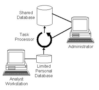
Note that when viewing data, the Analyst workstation communicates directly with the shared database, and does not go through the Task Processor.
